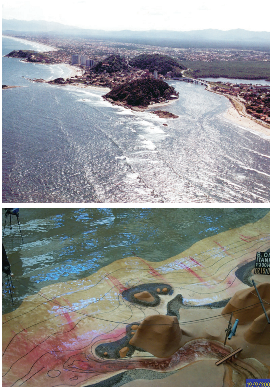
Figure 6. Aerial view of Itanhaém Bar (SP) and dye injection tests in the wave basin.
