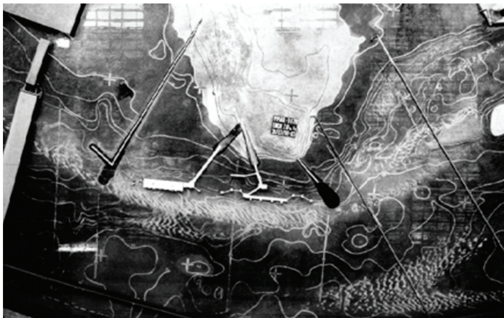
Figure 16. Sedimentological polystyrene tracer test of the Ponta da Madeira Harbour study.
