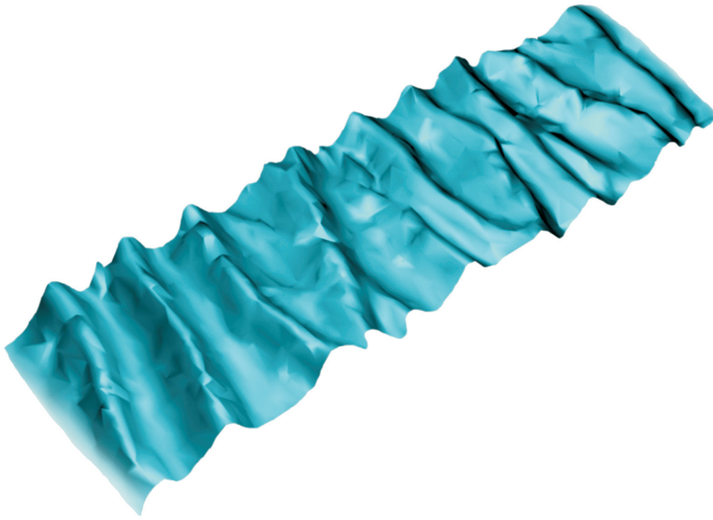
Figure 14. Sand waves formed in the Access Channel of Maranhão Harbour Area.
