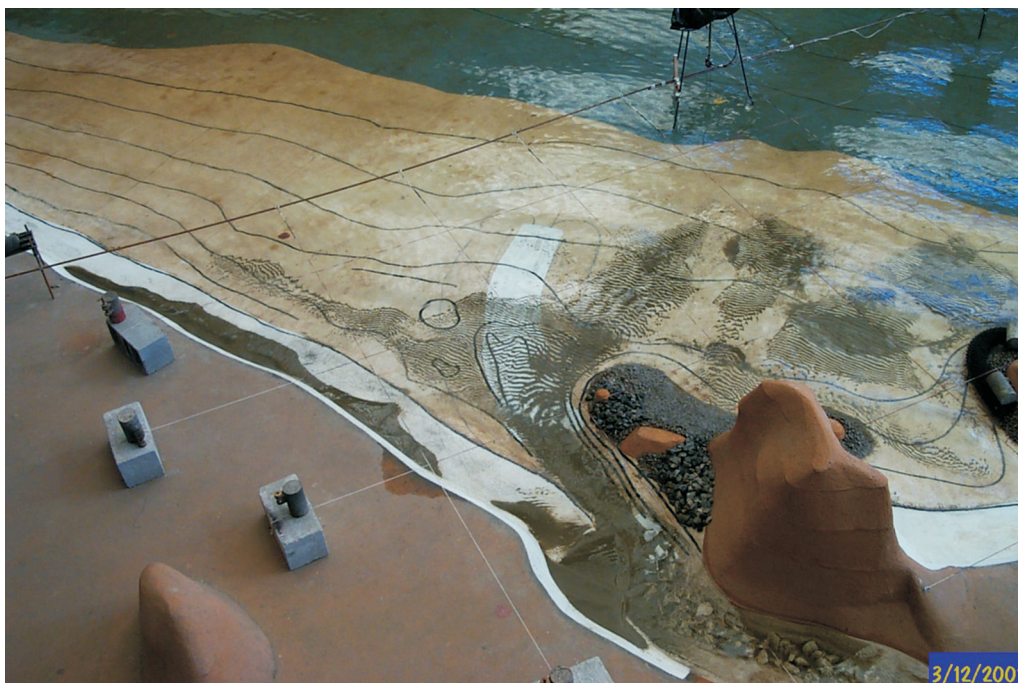
Figure 15. Sedimentological sand tracer test of the Itanhaém Bar Amelioration study.
