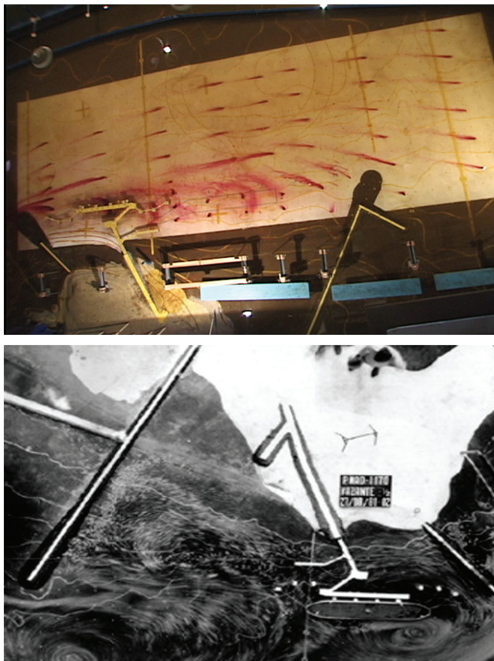
Figure 7. Dye injection and confettis tests in the Ponta da Madeira Harbour model.
