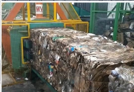
Pressed material to generate Waste Derived Fuel (CDR).
