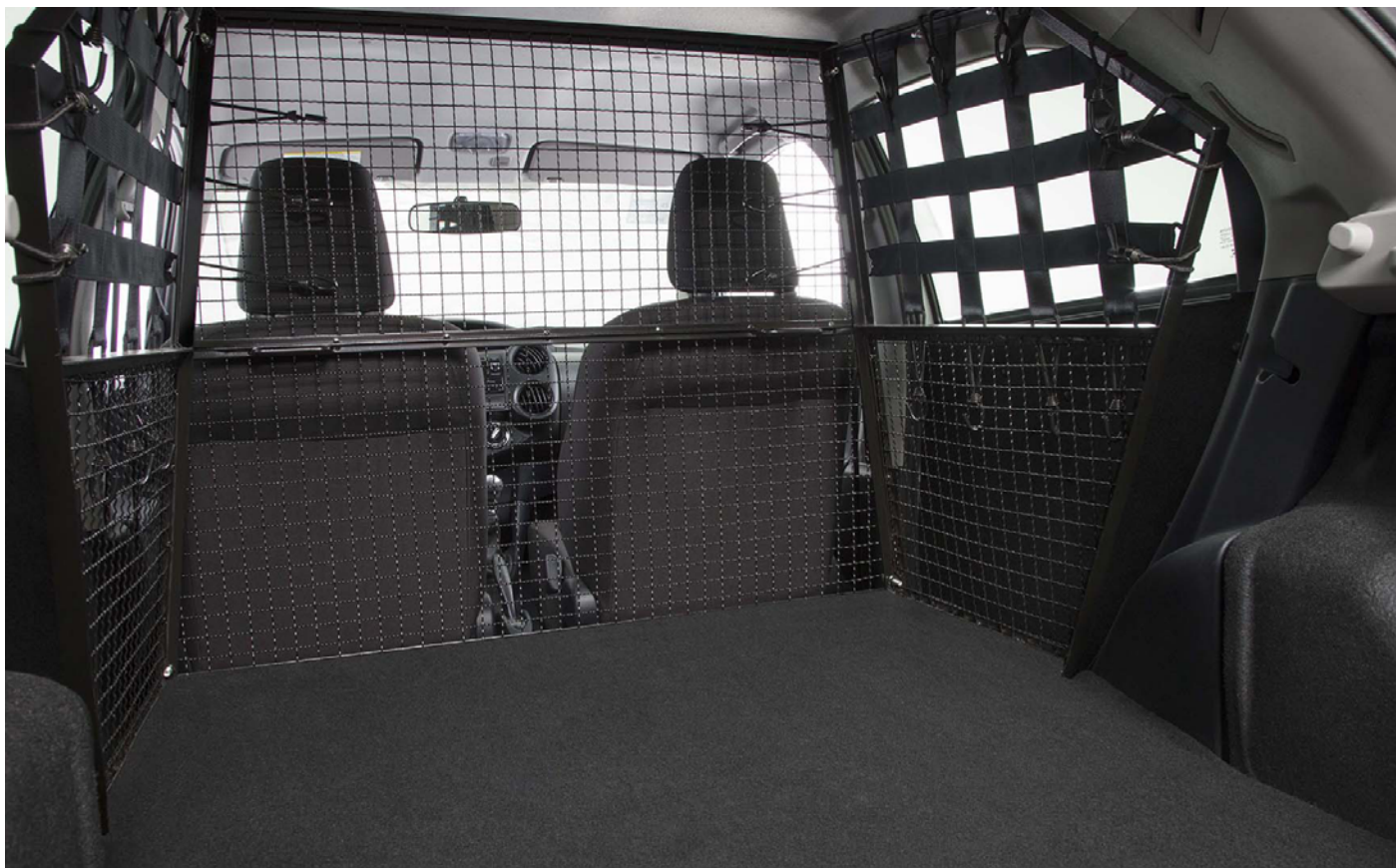
Safety net for the side windows made with leftover of seat belt.
